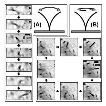
**Figure 4.** (A) Linear and (B) rotational actuation strokes of a single 500 nm rod with aspect ratio 50. Engineering specific magnetic geometries allows for a variety of rod beat patterns to be executed.
