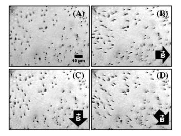
**Figure 5.** Rotational actuation of an array of 500 nm diameter rods with aspect ratios of 50. In (A), the rod array is pointing straight up, while in (B), (C), and (D), the arrows represent the planar direction of the applied magnetic field. Only about 0.1% of the entire sample array can be seen in these images. See Supporting Information for video (.mov) of the array actuation.
