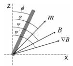
**Figure 6.** Angle and vector definitions used in deriving the rod bending theory. B is the applied magnetic field,  $\nabla B$  is the applied field gradient, and m is the rod's magnetic moment.
