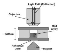
**Figure 3.** Experimental setup used to magnetically actuate rod arrays with simultaneous optical imaging. The thickness of the entire sample has been reduced to  $500~\mu m$  to allow high magnification microscopy from above while applying large magnetic forces from below.
