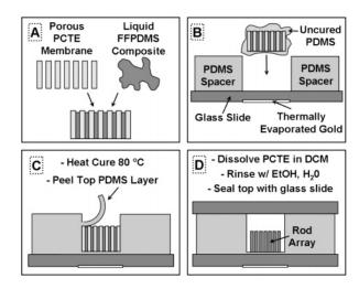
**Figure 1.** Cross-sectional view of the fabrication steps used to template magnetically actuated composite polymer rod arrays. Details in the text.
