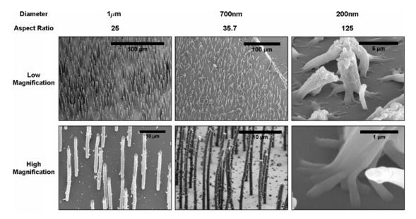
**Figure 2.** SEM images of various diameters of magnetically actuated rod arrays after being dried using supercritical CO<sub>2</sub>. In liquid environments, we are able to reliably fabricate and actuate rod arrays in the range of diameters pictured. However, as the diameter decreases, the rods become very flexible and supercritical drying without substantial rod collapse becomes increasingly difficult.
